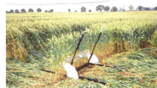
Figure 7 Lodgemeter being used in field trials
